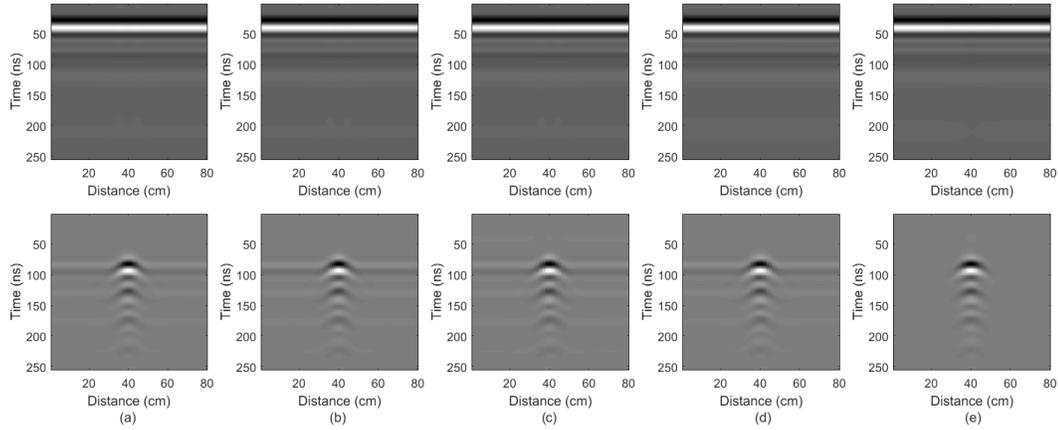
**Figure 5.** The results of the raw GPR image decomposition methods (first row clutter, second row target component) for flat surface ground a) SVD b) PCA c) ICA d) NMF e) RPCA.
