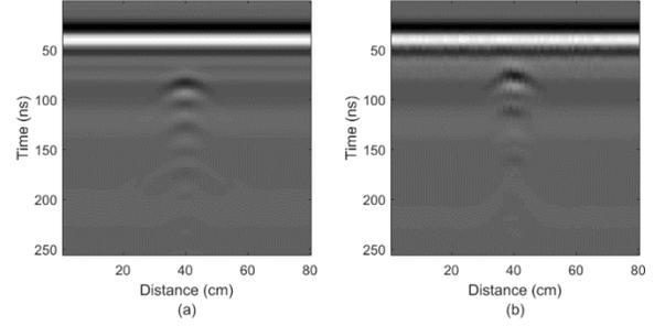
**Figure 4.** Sample raw GPR image from our simulated dataset a) flat and b) rough ground.
