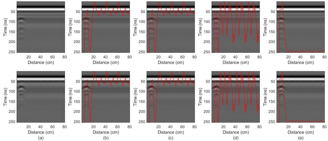
**Figure 9.** Energy based detection results (first row flat surface, second row rough surface) a) raw data, detection results b) LS c) regLS d)  $LS_{RPCA}$ , and e)  $regLS_{RPCA}$ .
