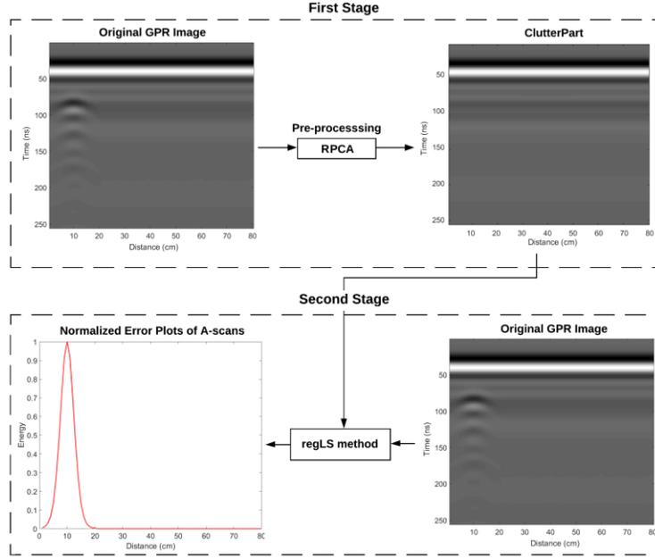
**Figure 2.** The two-stage block diagram of the proposed LS-based target detection.
