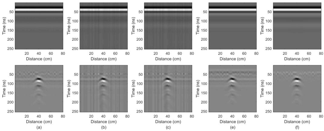
**Figure 6.** The results of the raw GPR image decomposition methods (first row clutter, second row target component) for rough surface ground a) SVD b) PCA c) ICA d) NMF e) RPCA.
