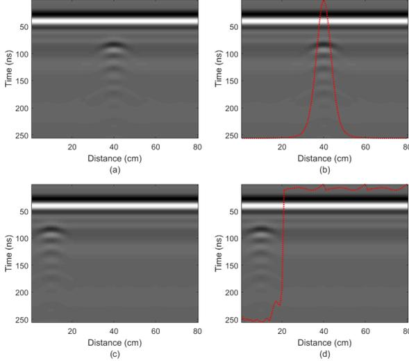
**Figure 1.** Sample raw GPR image with (a) target located in the middle, (b) LS detection result, (c) target located in the beginning, (d) LS detection result.
