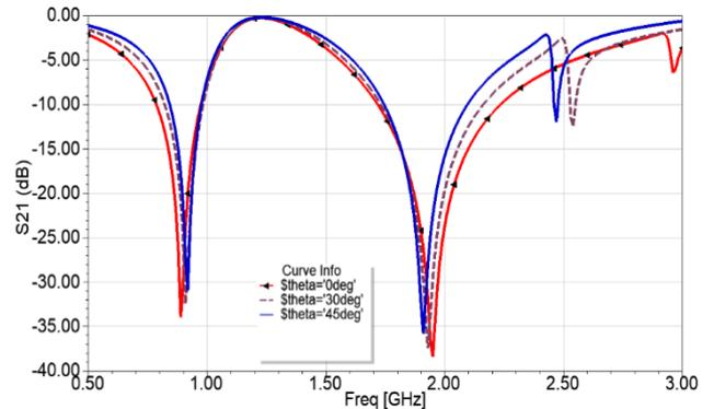
**Figure 8.**  $S_{21}$  frequency curves of the proposed FSS design (TM polarization,  $\theta=0^\circ$ ,  $30^\circ$  and  $45^\circ$ )
