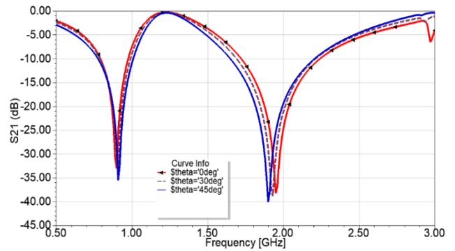
**Figure 7.**  $S_{21}$  frequency curves of the proposed FSS design (TE polarization,  $\theta=0^\circ$ ,  $30^\circ$  and  $45^\circ$ )
