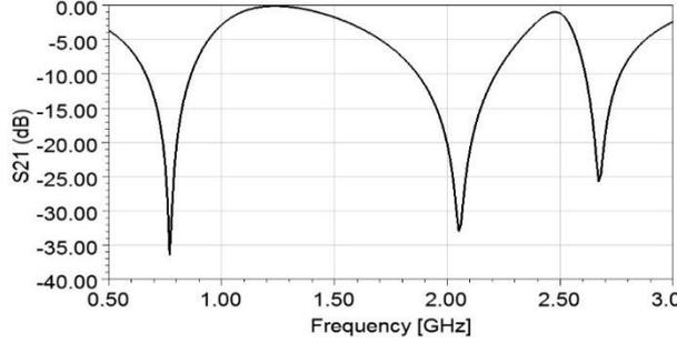
**Figure 5.**  $S_{21}$  frequency curve of the 2<sup>nd</sup> design stage (TE polarization,  $\theta=0^\circ$ )
