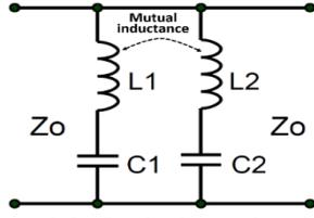
**Figure 1.** EC model of a dual stop-band FSS
