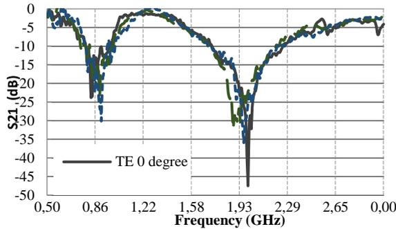
**Figure 10**  $S_{21}$  frequency curves of the proposed FSS design (TE polarization,  $\theta=0^\circ, 30^\circ$  and  $45^\circ$ )
