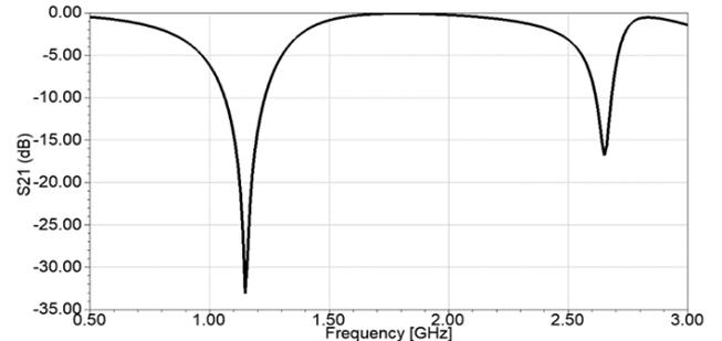
**Figure 4.**  $S_{21}$  frequency curve of the 1<sup>st</sup> design stage (TE polarization,  $\theta=0^\circ$ )
