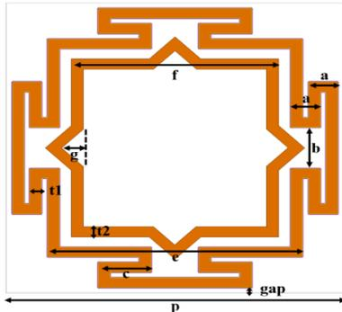
**Figure 6.** Proposed FSS geometry and its parameters
