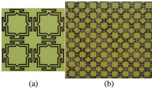
**Figure 9.** (a)  $4 \times 4$  array from the prototype of FSS. (b) Prototype of FSS
