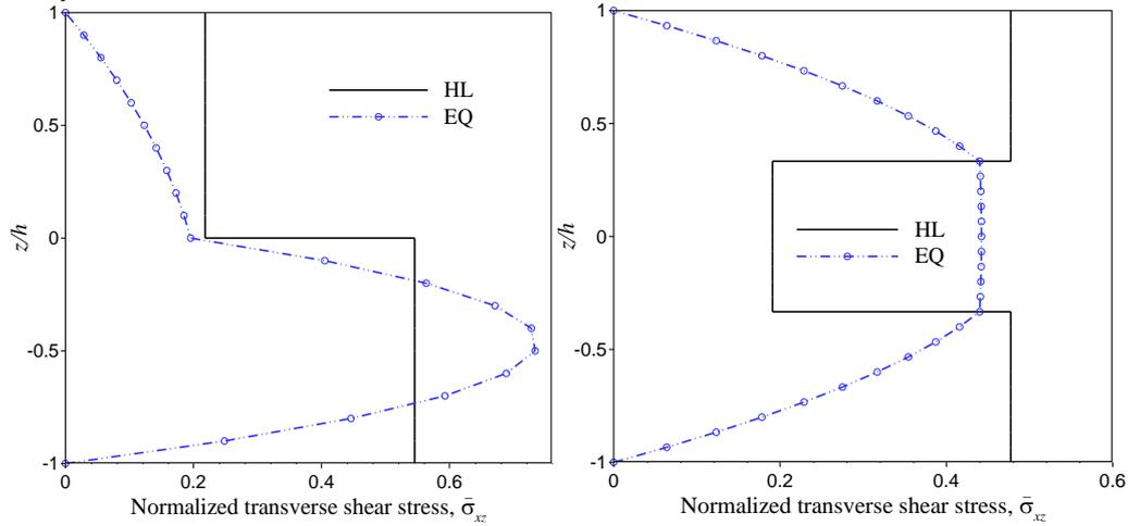
**Figure 5.** Variations of normalized transverse shear stress for simply supported (a) non-symmetric and (b) symmetric beams under sinusoidally distributed load ( $\rho = 10$ )
