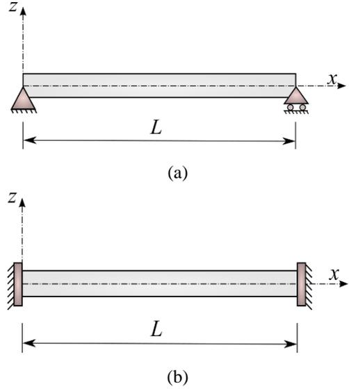
**Figure 3.** (a) Simply supported-simply supported (S-S) and (b) clamped-clamped (C-C) beams
