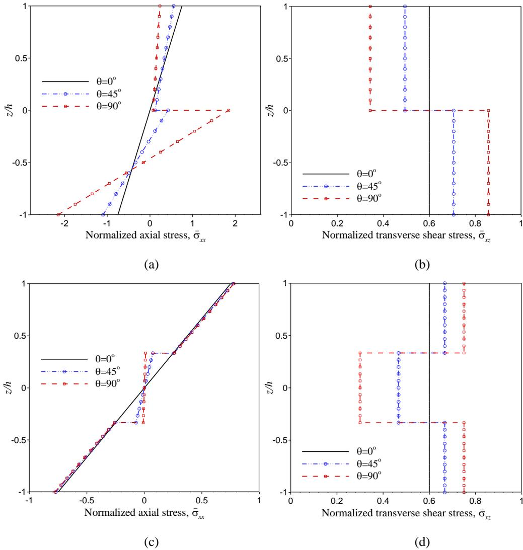
**Figure 4.** Variations of normalized (a) axial and (b) transverse shear stress for simply supported non-symmetric beam, (c) axial and (d) transverse shear stress for simply supported symmetric beam under uniformly distributed load ( $\rho = 10$ )
