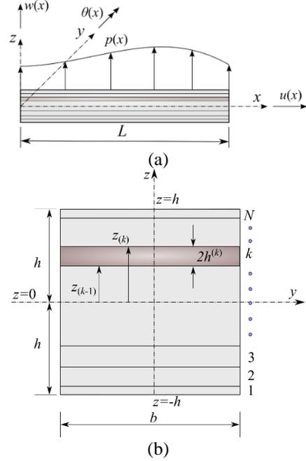
**Figure 2.** (a) Kinematics of TBT and (b) the cross-section of a beam
